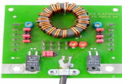
Figure 3.3-2: FEIG Antenna Tuning Board (Source FEIG [12]).
